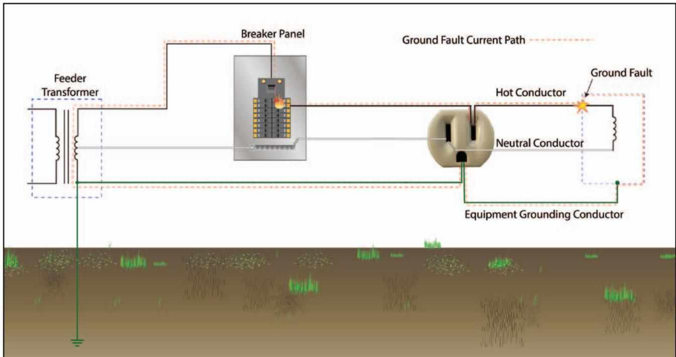
The purpose of that green equipment grounding conductor (EGC) is to establish “an effective ground-fault current path” in the event of a short circuit to the chassis of the equipment, which we call a “ground fault” even though it’s completely unrelated to the earth.
