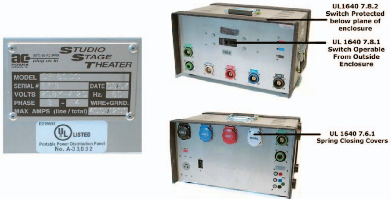
Figure 4 – Some of the UL1640 criteria to which manufacturers conform
