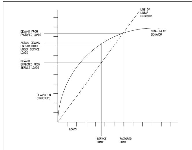
With ASD, the engineer designs for the actual loads that the structure is expected to see. That way, the demands that will be placed on the structure are correct and the designer can then apply the appropriate factor of safety.
