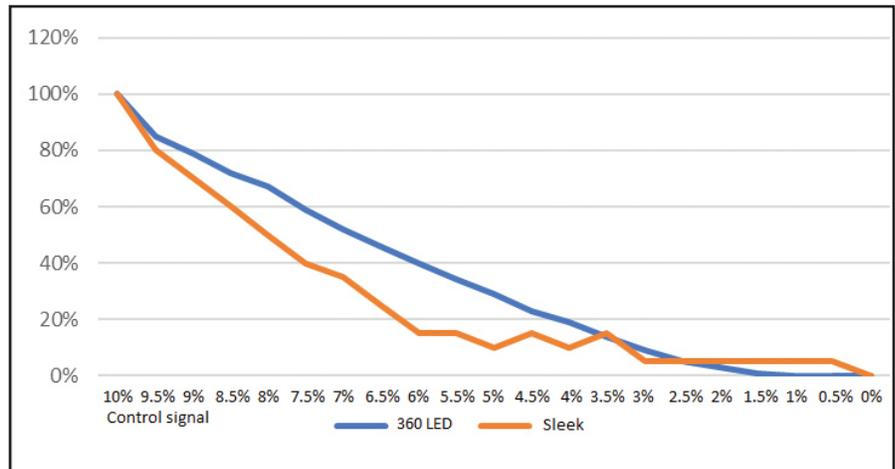
The low-end dimming outputs of the two luminaires, when plotted on the same graph, show significant differences. Both appeared to dim smoothly; the bobbles in the Sleek curve are reading differences of one or two lux, down at the level of noise. Not shown on this chart is that 0% for the Sleek unit was reached at about 44 V, while the 360 LED unit did not go black until below 24 V.
