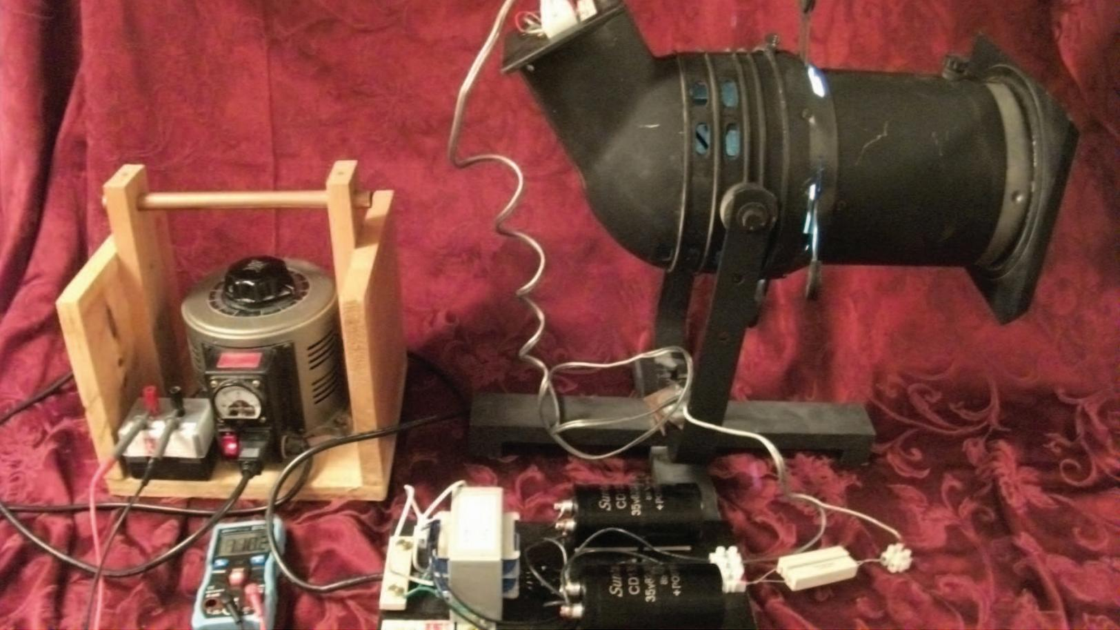
The LED luminaire based on an Altman 360 used a simple power supply to deliver DC power from an autotransformer.
