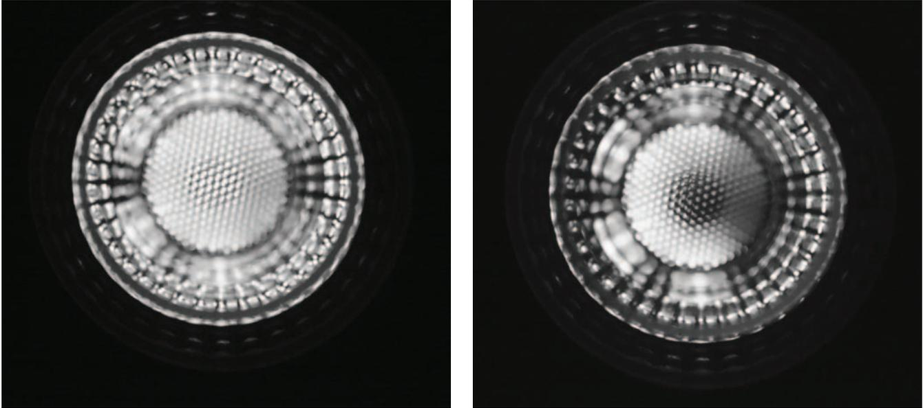
The Xerox copier lens could project an image of the Sleek LED PAR 20 face. It was fully illuminated when run at full, but parts of it dimmed out as I reduced power to it.
