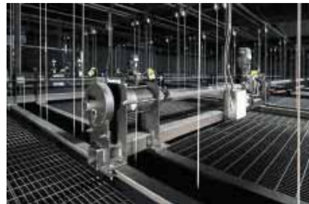
Figure 2 – Example rope design for a high-speed point hoist
