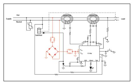
A schematic diagram of a GFCI shows the components, including an integrated circuit chip, which requires a supply voltage to operate (shown in red). If the GFCI is connected to the output of a dimmer, the supply voltage can be dimmed to the point that it drops low enough that the IC chip stops working. If the dimmer is connected to the output of the GFCI, the supply voltage for the GFCI is maintained throughout the dimming curve.
