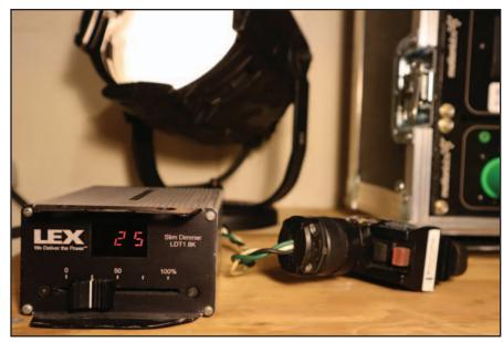
A portable GFCI (right) can supply enough power to protect single-channel dimmers, like the Lex Slimmer Dimmer, and smaller dimmer packs, like the Leprecon ULD series dimmers.
