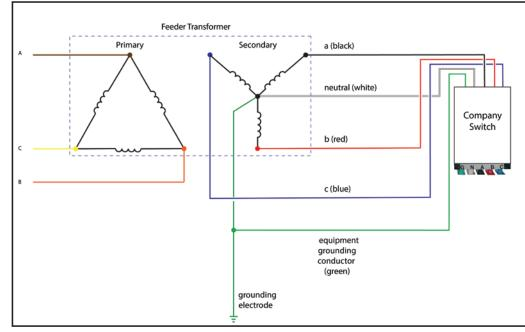
Grounding is the practice of connecting the neutral point of the electrical system to the earth through a grounding electrode. The same or similar terminology (ground or grounding) is used to describe the green (or green with a yellow stripe) conductor found in the power cable of all of our equipment.
