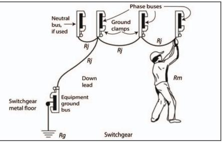
Figure 4 – If you can de-energize electrical equipment for inspection, it should be locked out, tested to ensure that it is de-energized, and it should be grounded to protect against induced voltage, re-energizing, lightning strikes, stored charges, or any other inadvertent re-energizing of the equipment.
