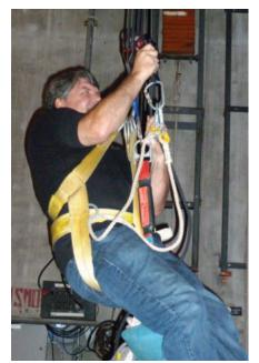
A "rescue cradle" with a block and fall are used to allow a single rescuer to ascend to the victim and then lower them to the ground.
